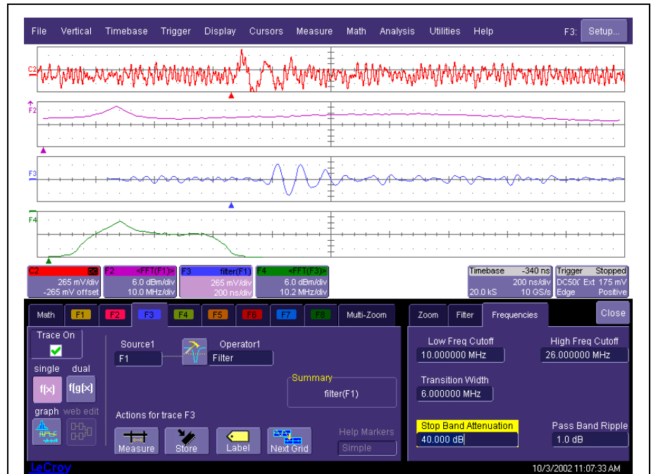
Figure 5 Use of a band pass filter to increase signal to noise ratio and recover a signal from broadband noise.
